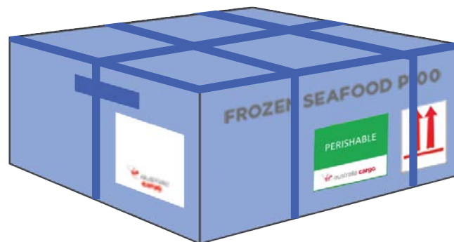
Example of labelling and marking of a package containing seafood, cooled using wet ice
