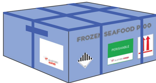
Example of labelling and marking of a package containing seafood, non-dangerous products cooled using dry ice.
