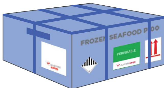
Example of labelling and marking of a package containing seafood, non-dangerous products cooled using dry ice.
